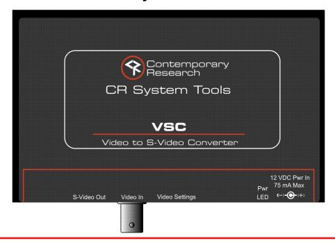
The VSC Video to S-Video Converter delivers high-quality S-Video signals from a composite NTSC video input. Employing technology developed for the popular 232-STS S-Video TV Tuner, the VSC features digital 2-D adaptive Y/C separation for superior S-Video performance.
